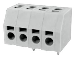
PCB spring terminal block Rated current: 8 A Rated voltage: 300 V Wire range: 20-16 AWG Pitch: 5.0 mm Mounting: Wave soldering
