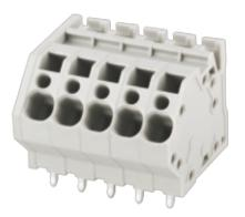
PCB spring terminal block Rated current: 20 A Rated voltage: 300 V Wire range: 28-12 AWG Pitch: 5.0 mm Mounting: Wave soldering
