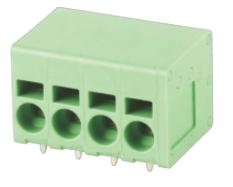
PCB spring terminal block Rated current: 20 A Rated voltage: 300 V Wire range: 24-12 AWG Pitch:5.0 mm Mounting: Wave soldering
