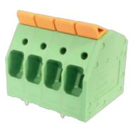
PCB spring terminal block Rated current: 41 A Rated voltage: 600 V Wire range: 24-8 AWG Pitch: 7.5 mm Mounting: Wave soldering
