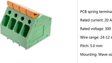
PCB spring terminal block Rated current: 20 A Rated voltage: 300 V Wire range: 24-12 AWG Mounting: Wave soldering
