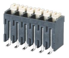
PCB spring terminal block Rated current: 10 A Rated voltage: 300 V Wire range: 24-16 AWG Pitch: 3.5 mm/3.81mm Mounting: Reflow soldering
