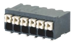
PCB spring terminal block Rated current: 10 A Rated voltage: 300 V Wire range: 24-16 AWG Pitch: 3.5 mm/3.81 mm Mounting: Reflow soldering
