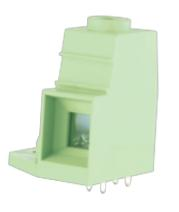
PCB terminal block Rated current: 115 A Rated voltage: 600 V Wire range: 20-2 AWG Pitch: 15.0 mm Mounting: Wave soldering
