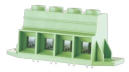
PCB terminal block Rated current: 115 A Rated voltage: 600 V Wire range: 20-2 AWG Pitch: 15.0 mm Mounting: Wave soldering
