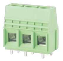
PCB terminal block Rated current: 65 A Rated voltage: 600 V Wire range: 20-6 AWG Pitch:10.16 mm Mounting: Wave soldering
