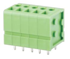
PCB terminal block Rated current: 20 A Rated voltage: 300 V Wire range: 26-12 AWG Pitch: 5.0 mm Mounting: Wave soldering
