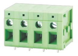
PCB terminal block Rated current: 20 A Rated voltage: 300 V Wire range: 26-12 AWG Pitch: 7.5 mm Mounting: Wave soldering
