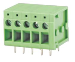
PCB terminal block Rated current: 20 A Rated voltage: 300 V Wire range: 26-12 AWG Pitch: 5.0 mm Mounting: Wave soldering
