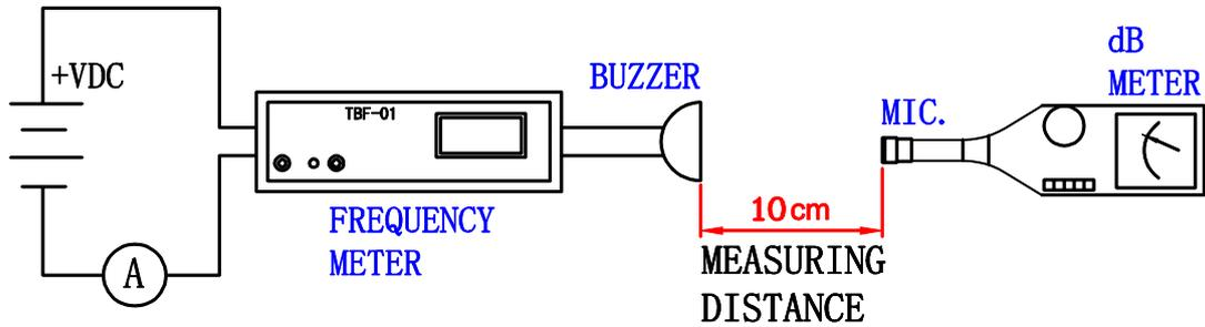
In the measuring test, buzzer is placed as follows:
