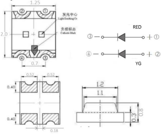
**Note:** Tolerance unless mentioned is ±0.1mm,Unit = mm.
