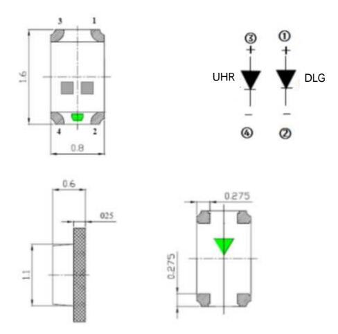
**Note:** Tolerance unless mentioned is  $\pm 0.1$ mm,Unit = mm.
