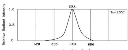
wavelength  $\lambda$  (nm) RELATIVE INTENSITY Vs. WAVELENGTH
