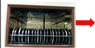
Correct way: material desiccant need to remove the bag, use the way of hanging baked
